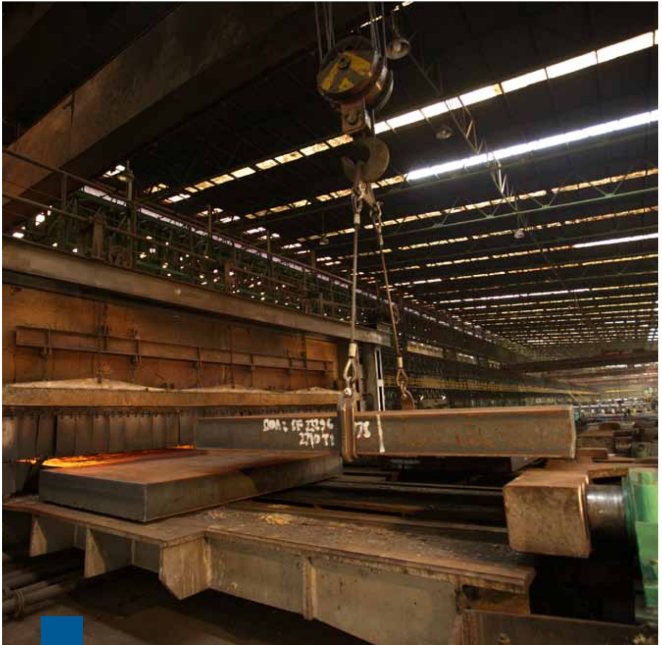
PROSES PEMASUKAN SLAB KE DAPUR PEMANAS PROCESS OF ENTERING SLAB INTO REHEATING FURNACE
