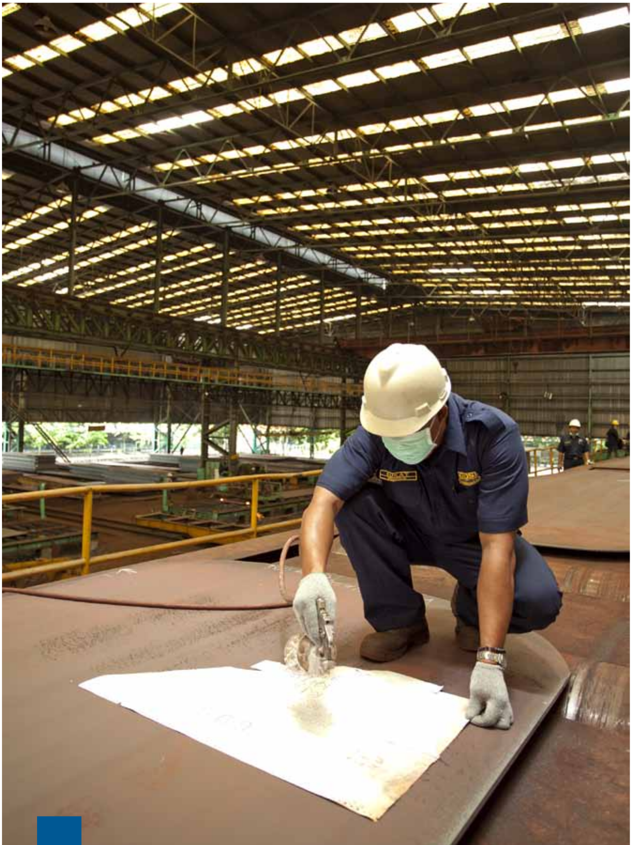
PROSES MARKING PLAT PLATE MARKING PROCESS
